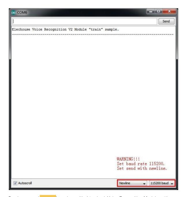
5. Send command settings(case insensitive) to check Voice Recognition Module settings.
