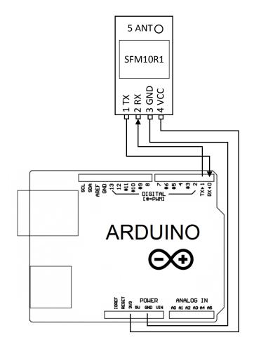
This is the simplest connection with the shortest code that is needed. After power supply connected to Arduino board message 0x01020304 will sent to Sigfox network.
