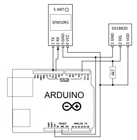
This image depicts connection of LPWAN Sigfox node to the Arduino for measuring temperature by sensor DS18B20. Communication between Arduino and Sigfox node is achieved by SoftwareSerial library (pins D10 and D11), therefore is hardware UART (pins D0 and D1) free for communication between Arduino and computer. Temperature sensor DS18B20 use OneWire bus that is initialized at pin D2.
